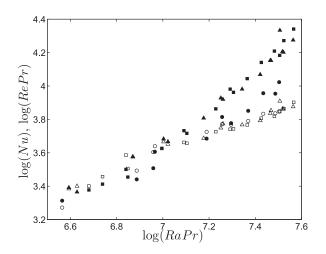
FIG. 3. Solid symbols: Nusselt number. Open symbols: Reynolds number. Circles:  $20 \degree C(Pr = 7)$ ; triangles:  $30 \degree C(Pr = 5.3)$ ; squares:  $40 \degree C(Pr = 4)$ .
