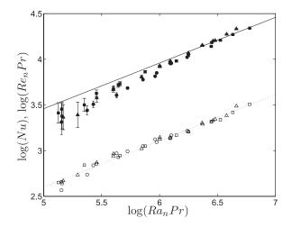
FIG. 4. With Re<sub>n</sub> and Ra<sub>n</sub> based on the coherence length  $L = \theta/2\beta$ , the experiments at different Prandtl merge. Same symbols as in Fig. 3. The dotted line corresponds to Re<sub>n</sub> Pr =  $1.14\sqrt{\text{Ra}_n \text{Pr}}$  and the solid one to Nu =  $9.1\sqrt{\text{Ra}_n \text{Pr}}$ .
