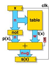
Fig. 3. Architecture of the seed generator.
