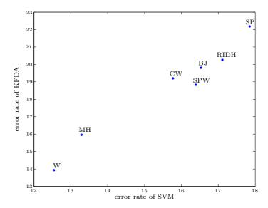
Fig. 4. Error rates of time-frequency-based SVM and KFDA using various distributions of the Cohen class: Wigner (W), smoothed pseudo-Wigner (SPW), Margenau-Hill (MH), Choï-Williams (CW), Born-Jordan (BJ), reduced-interference with Hanning window (RIDH) and spectrogram (SP). Same data as in Fig. 3.
