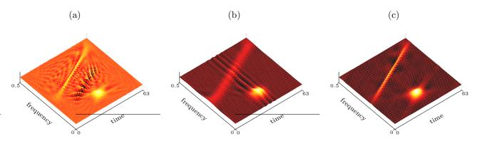
Fig. 1. First eigendistribution  $\Phi_1$  obtained using (a) Wigner-based KPCA, (b) Choï-Williams-based KPCA and (c) AOK algorithm applied to the Wigner-based KPCA result. The experiments were carried out using a collection of 1000 signals, each of length 64, consisting of a linear chirp and a Gaussian pulse in an additive white Gaussian noise with a standard deviation of 1.
