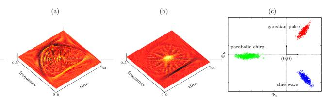
Fig. 5. The time-frequency patterns  $\Phi_a$  and  $\Phi_b$ , in (a) and (b) respectively, were extracted by Wigner-based GDA in a three-class classification problem involving sine waves, frequency-modulated waves with a parabolic modulation and Gaussian pulses embedded in noise. In (c), the training data are represented in the  $\Phi_a\Phi_b$  plane.
