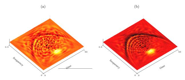
Fig. 3. Discriminant information extracted by (a) Wigner-based KFDA and (b) Wigner-based SVM. The experiments were carried out using two classes of 1000 signals, each of length 64, consisting of a frequency-modulated waves with a parabolic modulation and a Gaussian pulse, respectively, in an additive white Gaussian noise with a standard deviation of 2.2.
