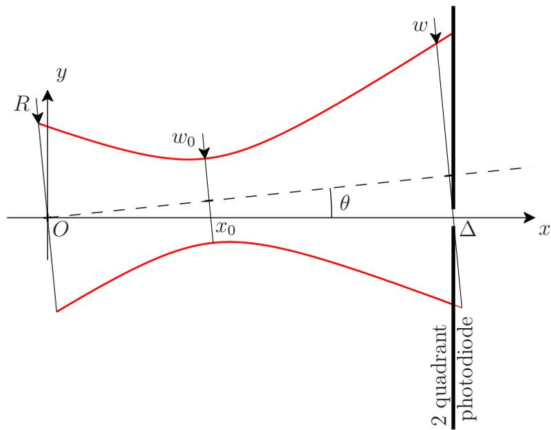
Figure 9: Principle of the optical lever technique: the incident beam illuminates a 2 quadrant photodiode, and for small deflections  $\theta$ , the difference between the intensities on the 2 segments is a linear function of  $\theta$ .
