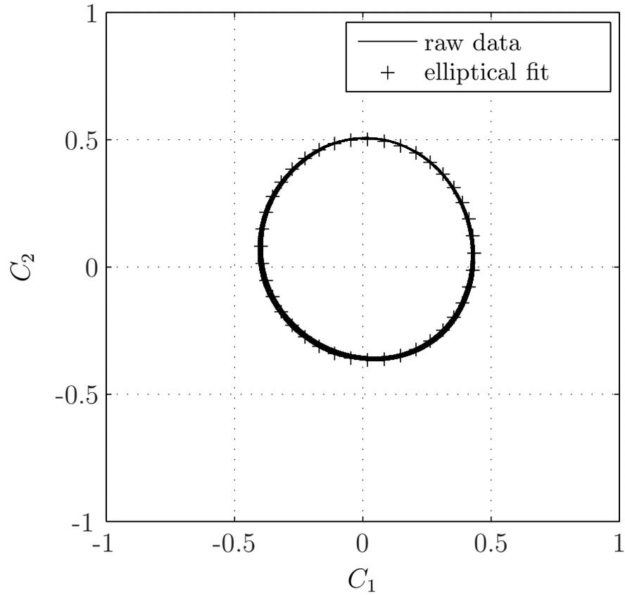
Figure 5: Due to experimental imprecisions, the measurement lays on a tilted ellipse in the  $C_1, C_2$  plane. These deviations to the  $C_{max}$  radius circle can easily be corrected [13]. We present the raw data to show that corrections are small anyway.
