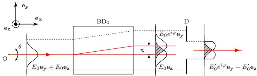
Figure 2: Experimental setup: measurement area. A collimated 6.6 mm He-Ne laser beam can be rotated around  $\mathbf{e}_z$  by means of a piezo driven kinematic mount. After passing through a parallel beam displacer (40 mm calcite prism,  $BD_0$ ), the 2 resulting crossed polarized rays present a phase shift  $\varphi$  dependent on the angle of incidence  $\theta$ . We limit the 2 beams to their overlapping part using a diaphragm (D), and analyze the emerging light ray into the analysis area.
