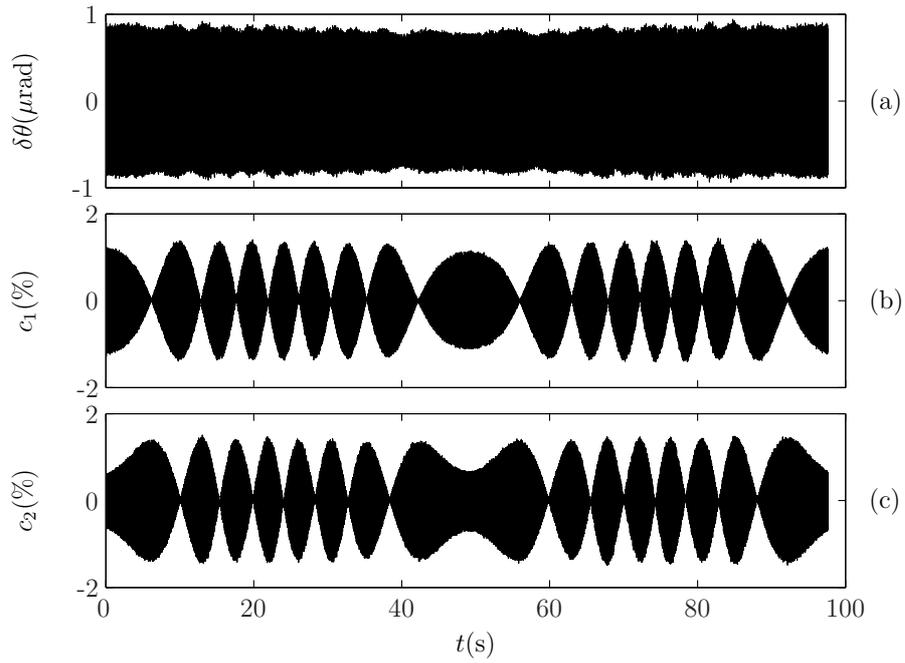
Figure 6: Fast evolution of the beam's angular position once the slow variation of Fig. 4 has been subtracted. (a) Fast angular displacement  $\delta\theta$  as function of the time. (b) and (c) Fast contrasts  $c_i$  of the two analyzing arms.
