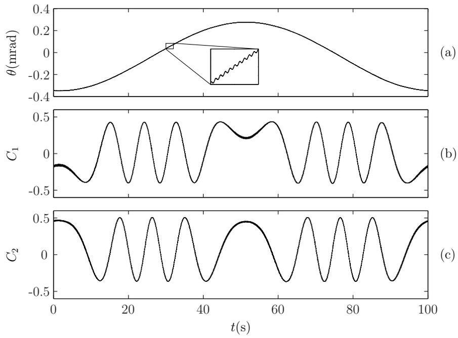
Figure 4: (a) Measured angular position  $\theta$  of the laser beam. The driving is the sum of two sinusoids : 0.5 mrad at 10 mHz and 1  $\mu$ rad at 10 Hz. (b) and (c) corresponding contrasts  $C_1$  and  $C_2$  of the two analyzing arms as a function of time.
