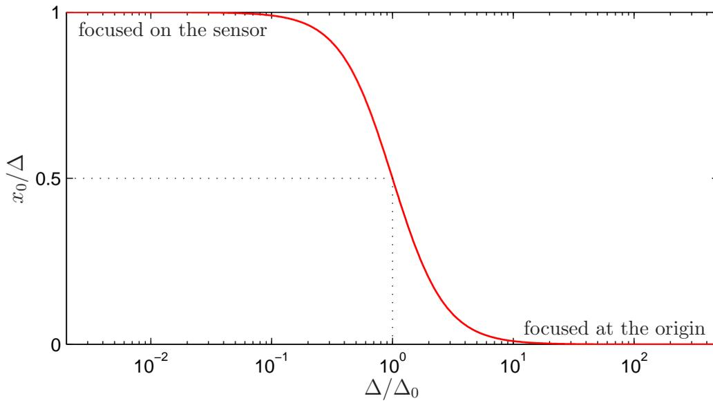
Figure 10: Optimal focalization of the beam to achieve best sensitivity in rotation measurement with a 2 quadrant detection. For large values of the distance between the sensor and the axis of rotation ( $\Delta \gg \Delta_0 = \pi R^2/\lambda$ ), one should focus the beam at the origin, whereas for small values of  $\Delta$  ( $\Delta \ll \Delta_0$ ) it should be focused on the 2 quadrant detector.
