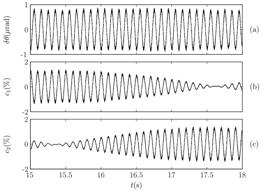
Figure 7: Zoom of Fig. 6: fast signals  $\delta\theta$  (a),  $c_1$  (b),  $c_2$  (c) around minimums of  $C_1$  and  $C_2$ . The reconstructed angular position  $\delta\theta$  is independent of the working point.
