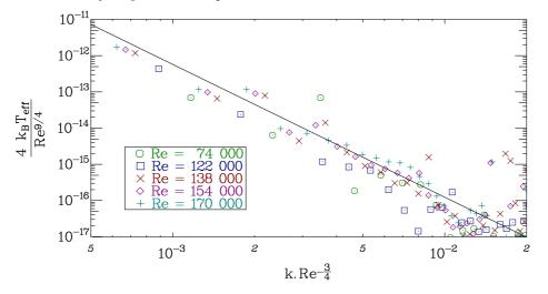
**Figure 4.** Spectrum of the FDR, labelled as *thermal agitation* per degree of freedom. Axis are rescaled with proper Reynolds number dependence, between 74000 and 170000. The size of the symbols represents the uncertainty in the determination of the maxima of the peaks. The solid line is a  $k^{-11/3}$  power-law given as an eye guide.
