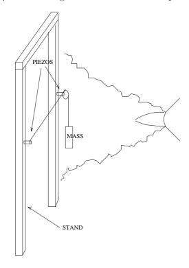
**Figure 1.** Eperimental setup: the thin steel wire is pulled across a turbulent air jet by a 4 Kg weight on a rigid stand. Piezoelectric transducers are in mecanical contact with the wire at each end.
