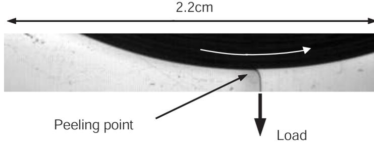
FIG. 4 – Image of the region near the peeling point ( $512 * 64$  pixel<sup>2</sup>).
