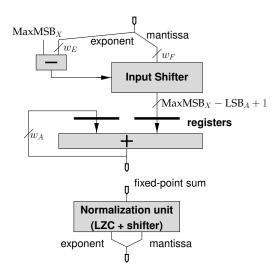
Figure 5: The proposed accumulator. Only the registers on the accumulator itself are shown, the rest of the design is combinatorial and can be pipelined arbitrarily.
