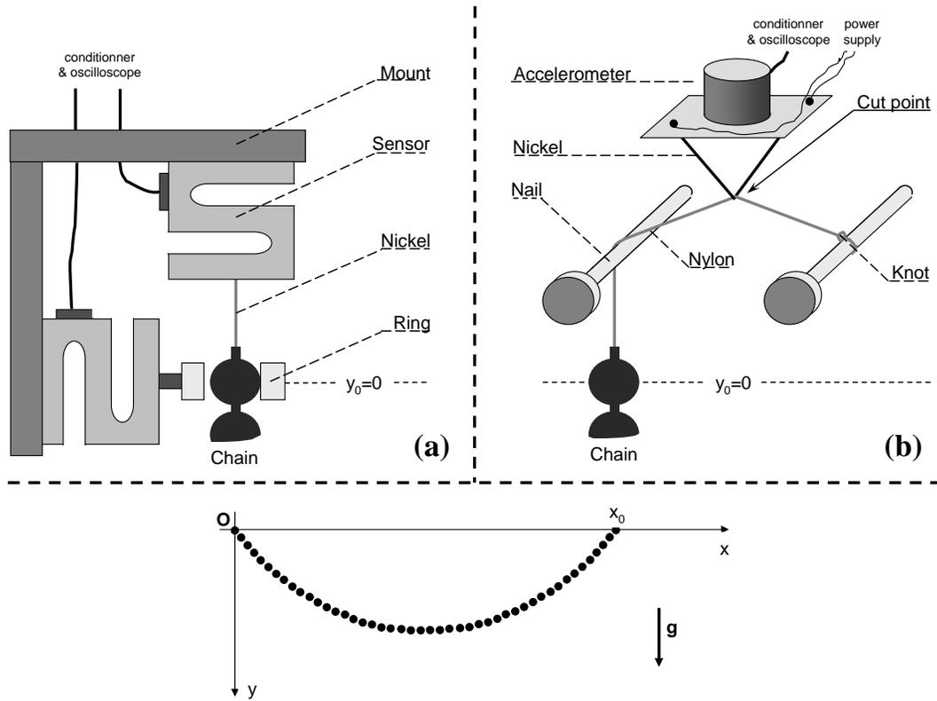
FIG. 1: **Sketch of the experimental setup.** The chain is initially stretched between two points having the same altitude  $y_0 = 0$  separated by the distance  $x_0$ . (a): Detail of the fastening in  $O$  ( $x = 0$ ), where the force is measured. (b): Detail of the fastening at  $x_0$ , where the chain is released.
