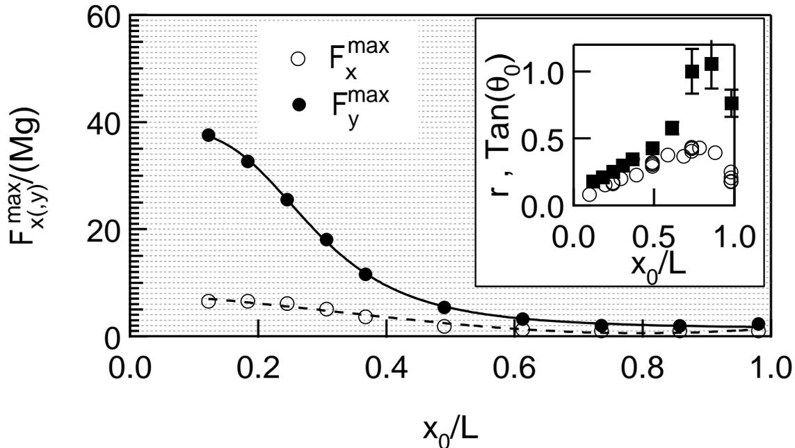
FIG. 4: **Maximum values of the force components.** The maximum values of the force components are reported in units of  $Mg$ , the total weight of the chain. The lines are polynomial interpolations helping to guide the eye. **Inset:**  $\tan(\theta_0)$  (Open circles) and  $r \equiv F_x^{max}/(F_y^{max} - Mg)$  (Full squares) as a function of  $x_0$  (Sec. III D).
