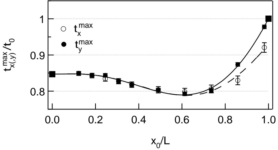
FIG. 3: **Times for the components of the force to reach their maximum value.** The times are reported in units of  $t_0$ , the characteristic time of the free fall over the distance  $L$ . The lines are polynomial interpolations helping to guide the eye. The full squares at  $x_0/L = 0$  and  $x_0/L = 1$  are theoretical limits of  $t_y^{max}$  (Sec. III B.)
