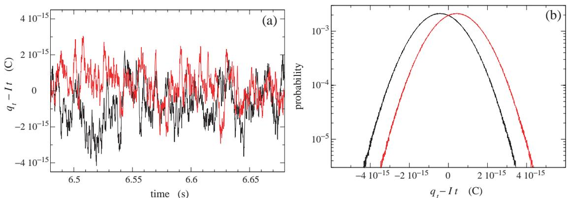
FIG. 6: (a) The time series of a typical path  $q_t - It$  for the Nyquist noise in the  $RC$  electric circuit driven by the current  $I$  (upper curve) and opposite current  $-I$  (lower curve) with  $I = 1.67 \times 10^{-13}$  A. (b) Gaussian probability distributions of the forward and backward experiments. The unit of the electric charge  $q_t - It$  is the Coulomb (C).
