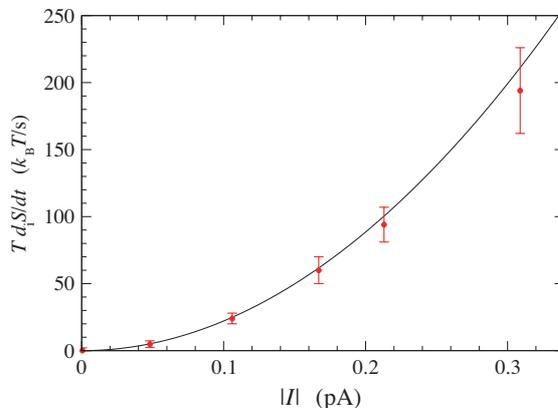
FIG. 8: Entropy production of the  $RC$  electric circuit versus the injected current  $I$ . The solid line is the Joule law,  $T d_i S/dt = RI^2$ . The dots are the results of Eq. (30). The equilibrium state is at zero current,  $I = 0$ , where the entropy production is observed to vanish.
