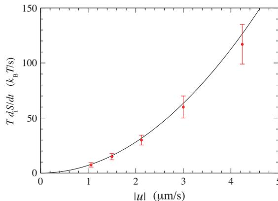
FIG. 3: Entropy production of the Brownian particle versus the driving speed  $u$ . The solid line is the well-known rate of dissipation given by Eq. (9). The dots depict the results of Eq. (30) calculated with the differences between the  $(\varepsilon, \tau)$ -entropies per unit time. The equilibrium state is at zero speed  $u = 0$  where the entropy production vanishes.
