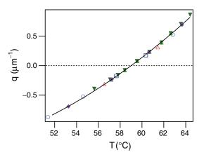
Fig. 4: Equilibrium twist as a function of temperature. The different symbols correspond to samples of different thicknesses  $(5, 6.8, 9 \text{ and } 20 \,\mu\text{m})$ .
