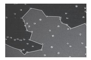
Fig. 3: Broken line separating an unwound zone (nematic phase, black) from a half-pitch twisted zone (grey). The line is pinned on the balls used to fix the sample thickness ( $d=20~\mu\mathrm{m}$ ,  $T=59.6~^{\circ}\mathrm{C}$ ).
