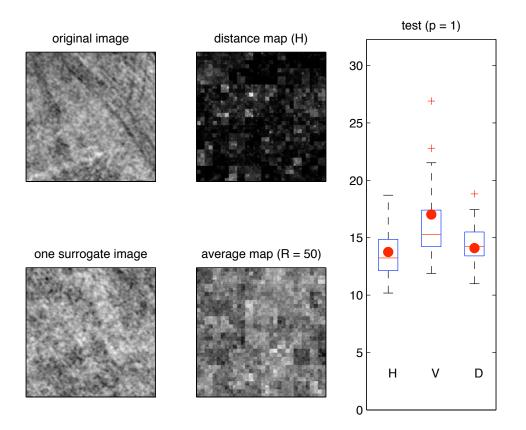
Figure 3. Same as in Fig. 2 when zooming in on a "stationary" region. At such a refined scale, stationarity is assessed by the test values for the actual scene (red dots) that lie within the corresponding distributions of the surrogates test values.
