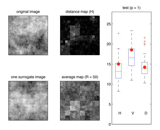
Figure 4. Same as in Fig. 2, but in the case of a 2D fractional Brownian motion with Hurst exponent H = 0.3. Within the considered framework, such a self-similar process appears as stationary.
