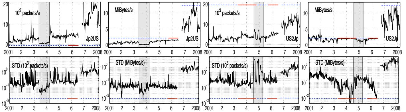
Fig. 1. **Throughput vs. years.** Top: Pkt and Byte throughputs. Bottom: Intraday variability (log of the standard deviation, computed from 1s time windows). Congestions are marked with solid lines (below for Pkt, at CAR bandwidth limitations for byte). Left: Jp2US; Right: US2Jp.
