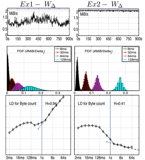
Fig. 3. **Traffic statistics under different conditions.** Aggregated ( $\Delta_0 = 1\text{ms}$ ) byte ( $W_\Delta$ ) count time series (top row); Marginal distributions (MD) for  $\Delta_j = 4, 32, 64, 128\text{ms}$ , both as empirical histograms (bars) and  $\Gamma$  fits (lines) (middle row); Logscale Diagrams (LD) (bottom row). *Ex1* (cols. 1): **B**-US2Jp, 2005/07/11, anomaly-free. *Ex2* (cols. 2): **B**-US2Jp, 2003/06/03, congestion.
