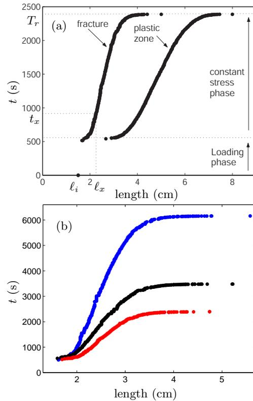
**Fig. 11.** (a) Time as a function of both the crack and plastic zone lengths for an imposed stress experiment ( $\ell_i = 1.5\text{cm}$ ,  $F = 900\text{N}$ ). We indicate the position of the inflexion point  $t_x$ ,  $\ell_x$  of the crack growth curve. (b) time as a function of  $\ell$  for three experiments performed with the same experimental conditions ( $\ell_i = 1.5\text{cm}$ ,  $F = 900\text{N}$ ).
