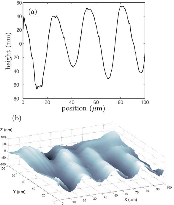
**Fig. 9.** (a) AFM profile of the plastic zone surface perpendicularly to the striations, (b) AFM three dimensional plot of a plastic zone surface, for a crack tip plastic zone in a  $125 \mu\text{m}$  thick film.
