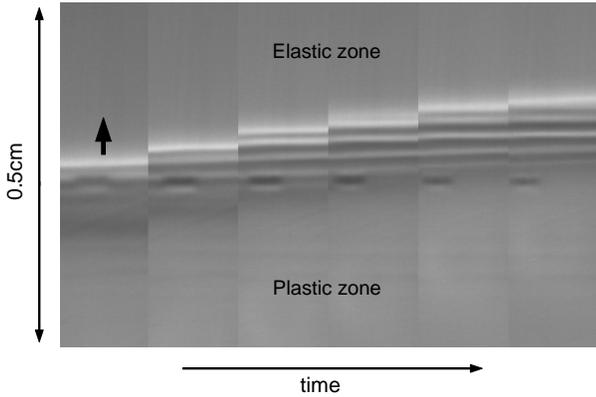
**Fig. 10.** Spatiotemporal microscopic image of the elastic-plastic frontier area during a creep experiment in a  $125\mu\text{m}$  thick polycarbonate strip. This figure shows the in situ formation of the surface oscillations inside the frontier, i.e. the shoulder of the necking instability, as it moves.
