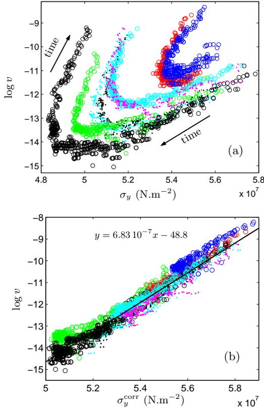
**Fig. 16.** Natural logarithm of the instantaneous crack growth velocity as a function of (a) the Dugdale-Barenblatt stress, (b) the corrected Dugdale-Barenblatt stress  $\sigma_y^{\text{corr}}$  according to Eq. (11) for eight experiments performed with various experimental conditions ( $\ell_i = 1.5, 2, 3\text{cm}$  and  $2.9 < \sigma < 3.8 \cdot 10^7 \text{N.m}^{-2}$ ). In Fig. (b), the black line is the result of a linear data fit.
