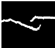
FIG. 5 – Close-up of a binary image of a fractured sample with d = 0\text{cm} .
