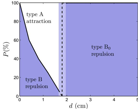
FIG. 8 – Percentage of samples for which the crack path are of type B (including the case  $B_0$ ). Experimentally, there is some uncertainty concerning the distance at which there is no more interactions between the two crack lines. This is schematically shown by the dotted line and lighter color band around  $d = 1.8\text{cm}$ .
