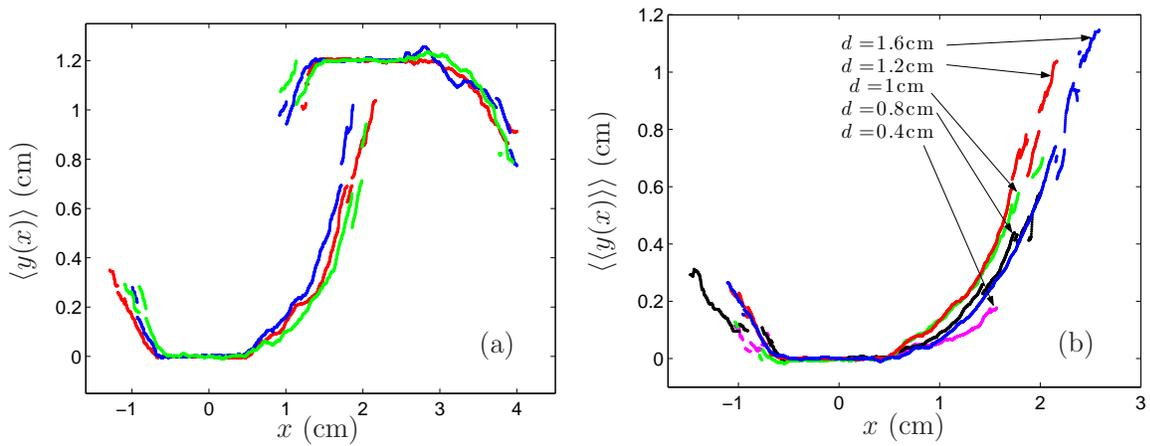
FIG. 9 – (a) Average crack profile  $\langle y(x) \rangle$  for three samples with  $d = 1.2\text{cm}$  and (b) average crack profile  $\langle\langle y(x) \rangle\rangle$  for five values of  $d$ , for experiments with a type A behavior.
