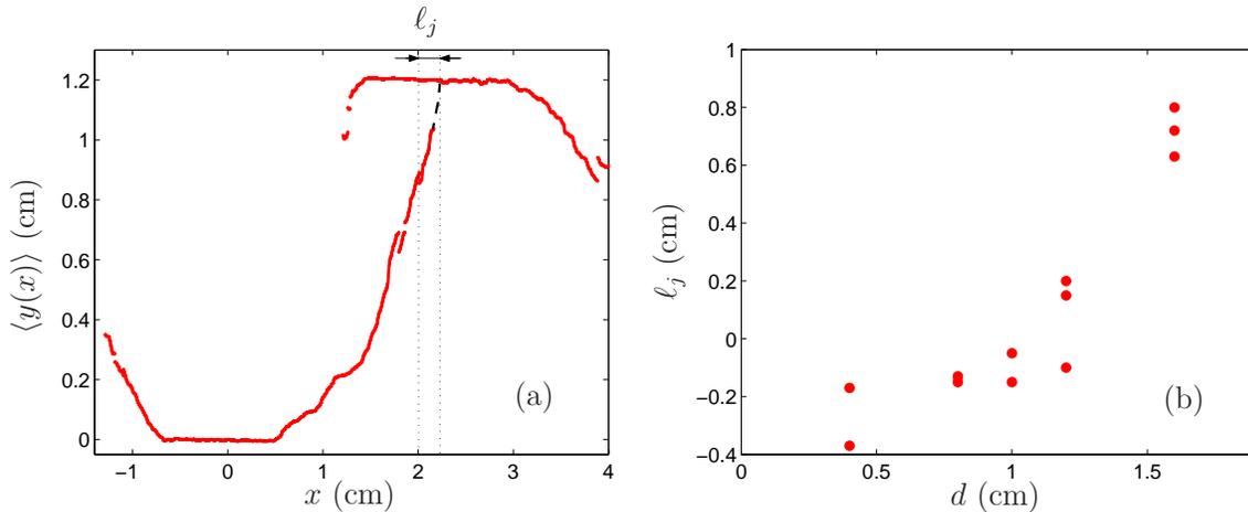
FIG. 10 – (a) Average crack profile  $\langle y(x) \rangle$  for a sample with  $d = 1.2\text{cm}$  and its extension allowing to define  $\ell_j$  and (b) distance  $\ell_j$  as a function of the spacing  $d$  between initial crack lines, for experiments with a type A behavior. Each point corresponds to one experiment.
