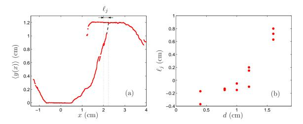
FIG. 10 – (a) Average crack profile  $\langle y(x) \rangle$  for a sample with d = 1.2cm and its extension allowing to define  $\ell_j$  and (b) distance  $\ell_j$  as a function of the spacing d between initial crack lines, for experiments with a type A behavior. Each point corresponds to one experiment.
