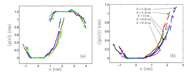
FIG. 9 – (a) Average crack profile  $\langle y(x) \rangle$  for three samples with d = 1.2cm and (b) average crack profile  $\langle \langle y(x) \rangle \rangle$  for five values of d, for experiments with a type A behavior.
