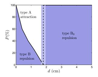
FIG. 8 – Percentage of samples for which the crack path are of type B (including the case  $B_0$ ). Experimentally, there is some uncertainty concerning the distance at which there is no more interactions between the two crack lines. This is schematically shown by the dotted line and lighter color band around d = 1.8cm.
