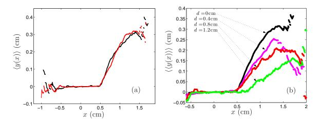
FIG. 11 – Paths of repelled cracks (type B). (a) Average crack profile  $\langle y(x) \rangle$  for two samples with d = 1 cm, and (b) average crack profile  $\langle \langle y(x) \rangle \rangle$  for four value of d.
