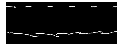
FIG. 7 – Binary image of a fractured sample with d = 5 cm.
