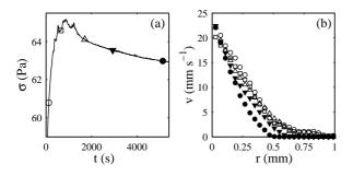
FIG. 1: Flow behavior in a rough Couette cell after a constant shear rate  $\dot{\gamma}=25\,\mathrm{s}^{-1}$  is imposed at  $t=0\,\mathrm{s}$ . (a) Stress response  $\sigma$  vs time t. (b) Velocity profiles v(r) at  $t=123\,\mathrm{s}$  (o), 653 s ( $\square$ ), 1702 s ( $\triangle$ ), 2931 s ( $\blacktriangledown$ ), and 5137 s ( $\bullet$ ). r is the radial distance from the inner rotating cylinder. Error bars are of the order of the marker size.
