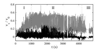
FIG. 3: Normalized apparent slip velocities  $v_s/v_0$  in the smooth geometry derived from linear fits of the velocity profiles over 0.2 mm from the stator (black) and from the rotor (grey), where  $v_0$  is the rotor velocity.
