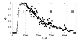
FIG. 5: Fraction  $\Phi$  of solidlike velocity profiles measured within a constant time window of 50 s during the experiment shown in Fig. 2. A velocity profile is counted as "solidlike" when the local shear rate in the middle of the gap is smaller than the threshold value 8 s<sup>-1</sup>. The thick line is the best exponential fit of  $\Phi(t)$  over regime II which yields a characteristic relaxation time of 1450 s.
