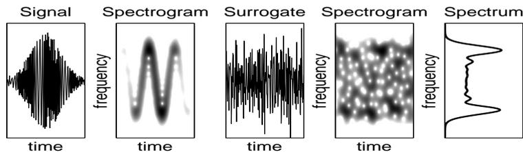
Figure 1: **Time-Frequency View of Surrogates.** Left to Right: a nonstationary signal; its spectrogram; a surrogate; the spectrogram of the surrogate; their common global (time-averaged) spectrum. One sees that the local frequency features, as compared to the global ones, will fluctuate more for the signals that for the surrogate which has a 'stationary' behavior (constant in time).
