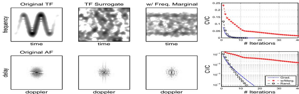
Figure 2: **Time-Frequency Surrogates: Examples and Convergence.** Spectrogram and Ambiguity function of a signal, one TF surrogate (positivity constraint) and one with also equality constraint in frequency marginal. Far right: Convergence criteria (sum of negative values divided by the sum of positive ones) vs.  $n$ .
