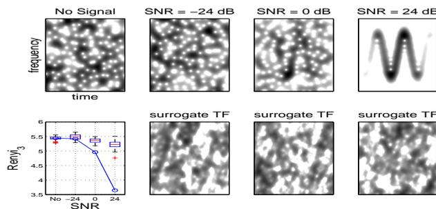
Figure 3: **Transient Detection.** A chirp is embedded in a white Gaussian noise with several SNR (-24, 0 and 24 dB); TFD of the signal and TF-surrogate with positivity constraint are shown. Bottom left: distribution of Rényi entropy of order 3 of the surrogates (box-plot) and value for the signal (circle); as this value is lower (if transient is significant, SNR 0 or higher), as compared to TF surrogates, this test detects transients.
