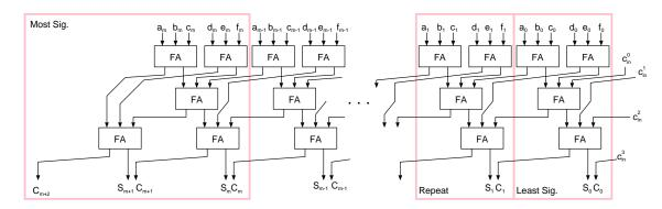
Fig. 5. [6:2] Adder module. The adder consists of three different slices: the least significant slice, which sums 6 arguments and takes 4 carry-ins, the repeat slice which sums 6 arguments and takes 4 lateral carries and produces 4 lateral carries to the subsequent slice, and the most significant slice.
