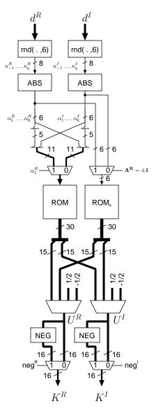
Fig. 3. TODO: update the figure. Prescaling ROM. The ABS block computes the absolute value of a two's complement number. Blocks rnd(., 6) round their argument to the sixth fractional position. NEG blocks negate their argument, a two's complement number.
