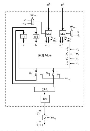
Fig. 6. Real recurrence module. Blocks  $\times 4$  shift their argument right by 2 binary places. Blocks MG compute  $\sigma$  times their argument using the  $\sigma_k^i$  decomposition discussed. The CPA module is a carry propagate adder which computes a short non-redundant estimate of the residual. The Sel module takes as argument this estimate and outputs the next quotient digit.
