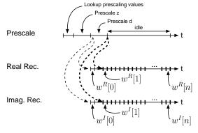
Fig. 2. Timing relationships between modules.
