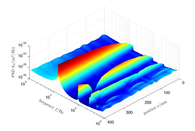
Figure 3: Power Spectrum Density (PSD)  $S_d$  of thermal noise induced deflexion as a function of position x along the cantilever and frequency f. The first 4 normal modes are clearly visible, with a vanishing amplitude toward the clamped extremity of the mechanical beam and the nodes of each mode. Another vibration peak with no nodes is also visible close to the third mode, it is attributed to the first mode in torsion, but is not studied in this letter.
