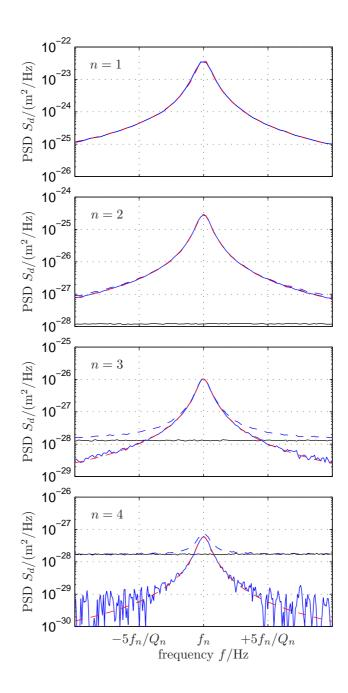
Figure 5: Power Spectrum Density (PSD)  $S_d$  of thermal noise induced deflexion measured close to the free end of the cantilever as a function of frequency f around each resonance  $f_n$ . We subtract from the raw measurement (dashed blue) the background noise (black) to estimate the mechanical noise of the cantilever (blue), then we perform a fit with a simple damped harmonic oscillator model (dashed red). For each plot, the horizontal scale spans  $\pm 10f_n/Q_n$  around  $f_n$ .
