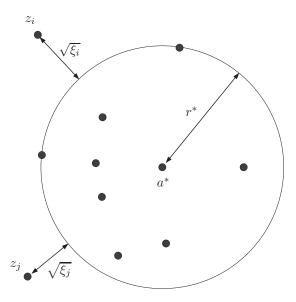
Fig. 6. Support vector data description algorithm
