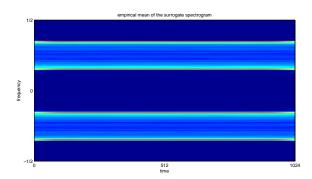
**Fig. 1**. Spectrogram of the FM signal (12) in the case where  $T = T_0$  (left), and empirical mean of the spectrogram of its surrogates (right).
