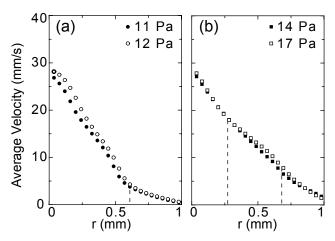
**Fig. 6.** Time-averaged velocity profiles for different shear stresses in the shear-thickening regime measured in the stress-controlled mode. r denotes the radial distance to the rotor; r = 0 at the rotor and r = 1 at the stator. Dotted vertical lines indicate position of the interface between the radial bands.
