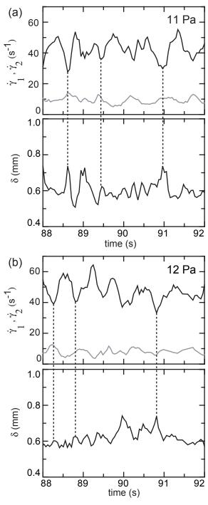
Fig. 7. Local shear rates  $(\dot{\gamma}_1, \dot{\gamma}_2)$  and position of the interface  $(\delta)$  as a function of time for (a) 11 Pa and (b) 12 Pa. The black and the gray lines on the top section of each figure correspond respectively to the highly sheared band  $(\dot{\gamma}_1)$  near the rotor and to the weakly sheared band  $(\dot{\gamma}_2)$  near the stator.
