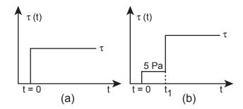
Fig. 4. Rheological test sequence used to measure velocity profiles. (a) Step stress method for shear stresses  $\tau \leq 10$  Pa and (b) Pre-shear and step stress method for shear stresses  $\tau > 10$  Pa;  $t_1 = 40$  s.
