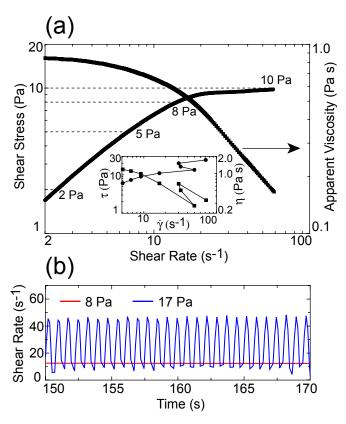
Fig. 3. Color online: (a) Flow curve of 40 mM CPyCl-NaSal solution ( $1 < \tau < 10$  Pa) with 1 wt% tracer particles recorded under controlled shear stress conditions. The inset shows the full flow curve including the shear thickening region. Horizontal dotted lines represent the stresses where the steady state UVP velocity profiles were recorded. (b) Transient shear rate signals below (8 Pa) and above (17 Pa) shear-thickening regime of flow.
