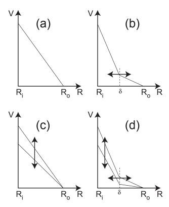
Fig. 1. Velocity profiles for (a) Newtonian fluid; (b) fluid showing radial shear-bands; (c) fluid with vorticity banding; and (d) fluid showing both the radial and vortity bands.  $R_i$  and  $R_o$  corresponds to the radii of inner (rotating) and outer (stationary) cylinders of the Couette cell while  $\delta$  is the boundary between the radial shear bands. The arrows indicate temporal fluctuations in the shear bands.
