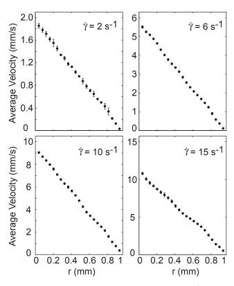
Fig. 10. Time-averaged velocity profiles for different shear rates in the Newtonian (2 and 6 s<sup>-1</sup>) and shear-thinning (10 and  $15 \text{ s}^{-1}$ ) regimes measured in the strain-controlled mode. Error bars correspond to the standard deviation of the local velocities and mainly account for temporal fluctuations in the velocity. r denotes the radial distance to the rotor; r = 0 at the rotor and r = 1 at the stator.
