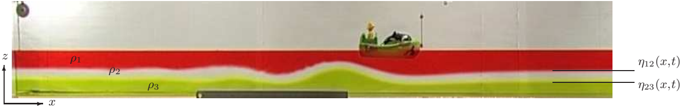
Fig. 14. Picture illustrating the dead-water phenomenon for a three-layer fluid.
