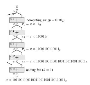
Fig. 1. Multiplication of a 24-bit mantissa by 7/5 (period  $p=0110_2,$  header h=1)
