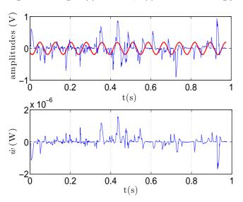
Fig. 3: Top: time-series of the imposed sine current ( $I \simeq 200 \mu A$ ), and the induced voltage. For homogeneity and comparison, both have been plotted in Volts: R~I(t) (bold), and for readability, e has been enlarged by a factor 100 (thin). Bottom: in the same time-scale, the corresponding energy flux  $\dot{w}(t)$  is plotted. The mean power given is  $<\dot{w}>\simeq 7.3~nW$ . The acceleration is  $a\simeq 56~{\rm ms}^{-2}$ .
