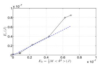
Fig. 9:  $E_c$  is plotted against the kinetic energy of the blade+rotor system:  $E_k = \frac{1}{2}M < \dot{\theta}^2 >$ . Dashed line is the best linear fit through 0. The acceleration of the vessel is varied between 41 ms<sup>-2</sup> and 59 ms<sup>-2</sup>, at constant frequency  $f_{\rm exc.} = 40\,{\rm Hz},\,I = 200\,\mu{\rm A}$  unchanged.
