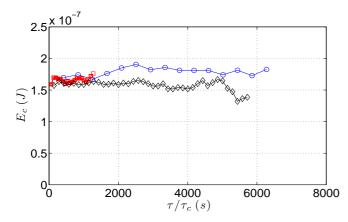
Fig. 8:  $E_c$  against  $\tau/\tau_c$ , for several values of the excitation current I ( $\Box$ : 1 mA,  $\Diamond$ : 700  $\mu$ A, and  $\bigcirc$ : 400  $\mu$ A), but the same acceleration:  $a=41\,\mathrm{ms}^{-2}$ .
