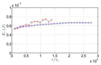
Fig. 7:  $E_c$  measured at  $I \simeq 200 \mu A$ , against  $\tau/\tau_c$ ,  $\tau_c$  being the correlation time of the process  $\dot{w}$ . The squares and circles refer to  $E_c$  measured according respectively to the first and second method.  $a=56\,\mathrm{ms}^{-2}$ .
