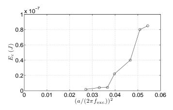
Fig. 10:  $E_c$  against  $(a/(2\pi f_{\rm exc.}))^2$ , for several values of the acceleration (between  $41\,{\rm ms}^{-2}$  and  $59\,{\rm ms}^{-2}$ ). The frequency  $f_{\rm exc.}=40\,{\rm Hz},\,I=200\,\mu{\rm A}$  unchanged.
