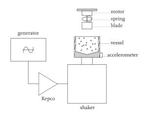
Fig. 1: The mechanical system is composed of a vibrating vessel with its driving, and the probing harmonic oscillator, pulled out for clarity.
