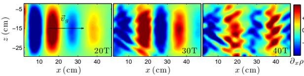
FIG. 1. (Color online) Snapshot of the horizontal density gradient (in  $\text{kg/m}^4$ ) obtained at  $t = 20T$ ,  $t = 30T$  and  $t = 40T$  with the parameters  $a = 0.5$  cm,  $\omega_0 = 0.95N$  and  $N = 0.822$   $\text{rad} \cdot \text{s}^{-1}$ . On the left-hand panel the direction of the group velocity,  $\vec{v}_g$ , is indicated. After  $20T$ , the primary wave has only reached a steady state in the first 20 cm from the generator (see Fig. 4).
