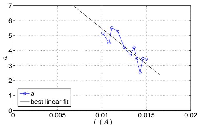
Fig. 7: The asymmetry coefficient  $a$  is obtained for each  $I$  by fitting the histogram with a generalised Gumbel distribution.  $a$  is plotted against the current  $I$ . A linear fitting is performed over the range available.
