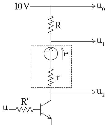
Fig. 2: The electrical sketch of the motor's command.
