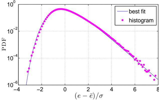
Fig. 4: A histogram of the centered and normalised induced voltage  $x(t) = (e(t) - \bar{e})/\sigma$  at fixed current  $I$  is plotted in semi-log axis (dots). The fitting is performed with a generalised Gumbel distribution (line). The best fit is obtained for  $a = 2.5$ .
