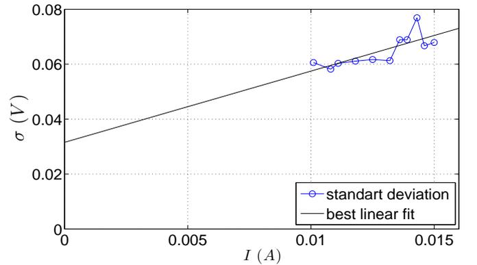
Fig. 6: The standard deviation of  $e$  at fixed current  $I$  is plotted against  $I$ . A linear fitting is performed over the range available.
