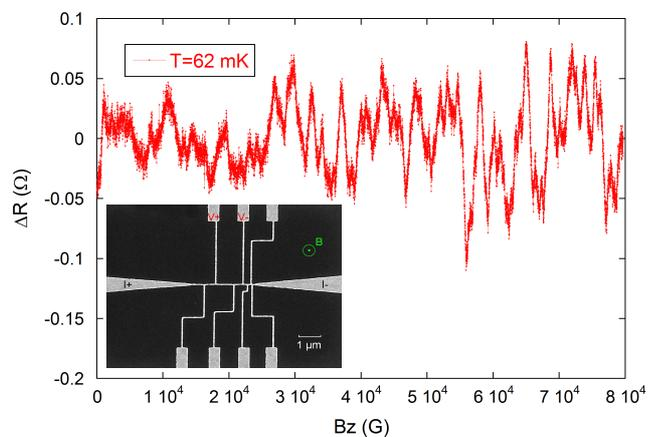
FIG. 1. (Color online) Magnetoresistance of a spin glass  $Ag$  sample implanted with 700 ppm of manganese. The magnetic field is applied perpendicularly to the sample. Insert: Scanning Electron Microscopy of the sample; current and voltage probes are indicated in red.
