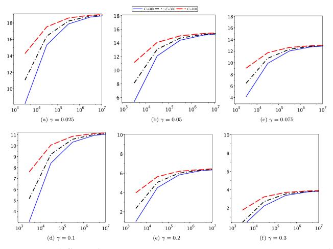
Figure 6: Gain (in % on y-axis) achieved, for optimal values of p and q over the base case p=q=1 when C=600 (10 minutes), C=300 (5 minutes) and C=100 ( $\approx 1.6$  minutes) as a function of the platform MTBF  $\mu$  (on log scale on x-axis) for six different V/C ratios.
