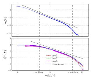
Figure 2: Top: Power Spectral Density of the experimental signal. The straight line corresponds to the K41 scaling. Bottom: entropy rate  $h_{\tau}^{(m)}$ , as a function of the scale  $(f = f_s/\tau)$  for different embedding dimensions  $m \in \{1, 2, 3\}$ . The blue curve corresponds to eq.(3) using the autocorrelation function. The straight line is a line of slope -1/3.
